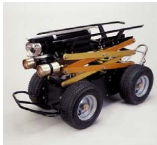
Storm Drain Tractor
