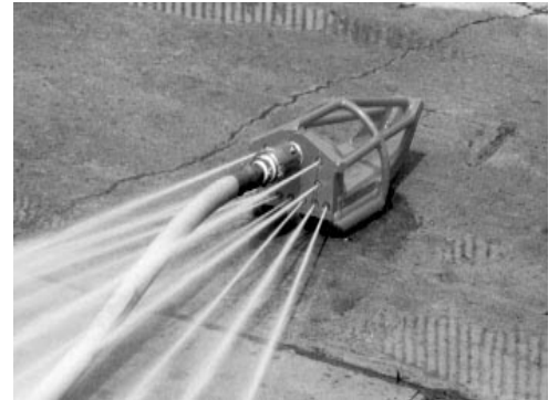
Boat Nozzle's unique structure controls nozzle position while sweeping main lines.
